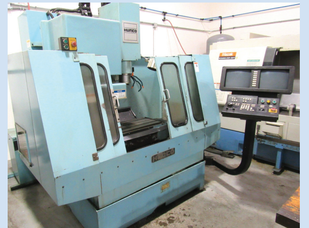
HURCO MODEL BMC-20 VERTICAL MACHINING CENTER
