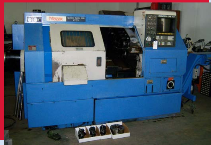
MAZAK MOD. QUICK TURN 10N ATC M/C 3-AXIS CNC TURNING/ MILLING CENTER
