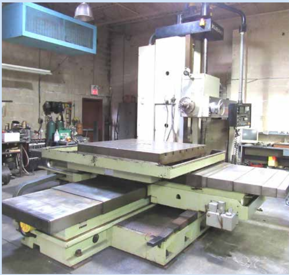
KURAKI Model KBT-11050DX 4.33" CNC Table-Type Horizontal Boring Mill with Fanuc 11M Control
