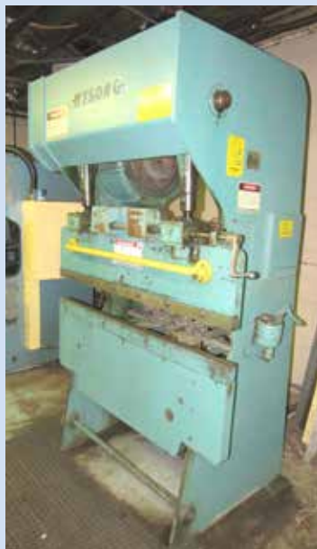
Wysong Model 2052 52" x 20 Ton Hydra- Mechanical Press Brake
