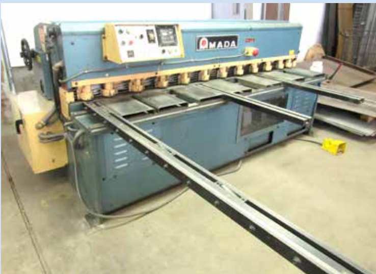
Amada Model S-2532 8' x 10 Ga. Hydraulic Power Squaring Shear
