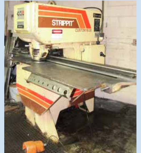
Strippit Custom 18/30 30 Ton Fabricating Punch w/Tooling
