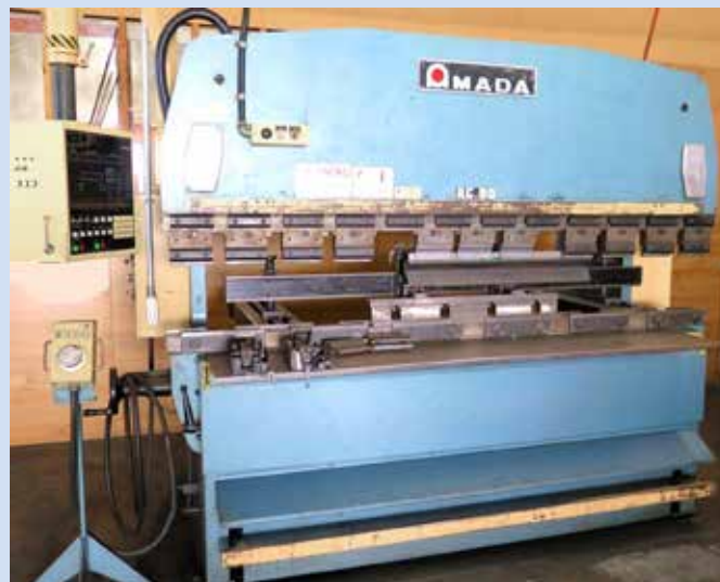
Amada Model RG-80 8' x 88-Ton CNC Press Brake w/Amada NC-9EX CNC Control
