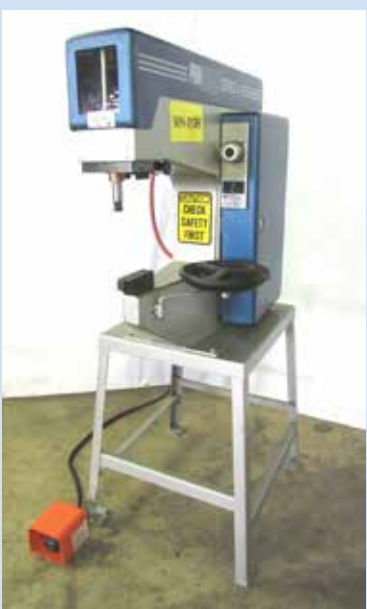
Pemsarter Series 4 6 Ton Pneumatic Insertion Press
